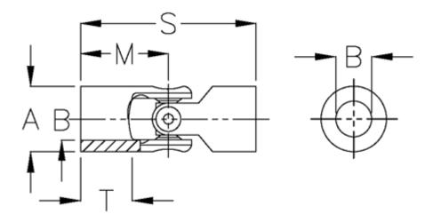
$\begin{array}{lll} A & = 40 \\ B \ H7 & = 25 \\ M & = 54 \\ MD \ max \ N \ m = 80 \\ s & = 108 \\ T & = 32 \\ \end{array}$
